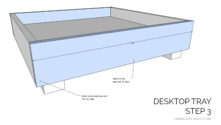
Step 3: Attach the long sides to the base and short sides using wood glue and ¾" pin nails.
