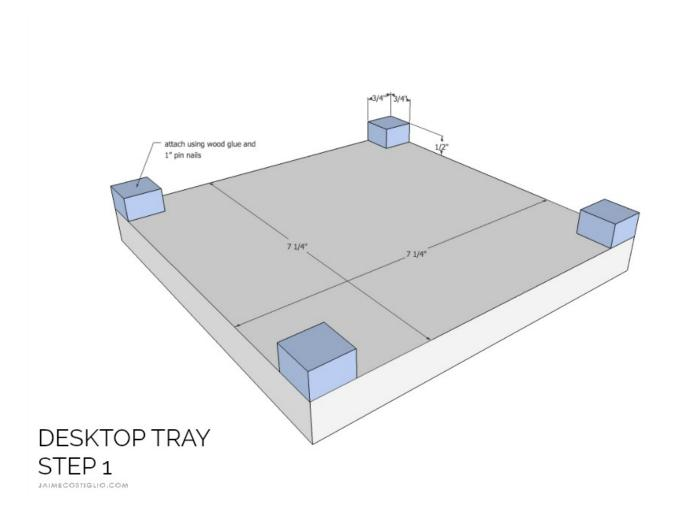
Step 1: Attach the feet to the base using wood glue and 1" pin nails.
