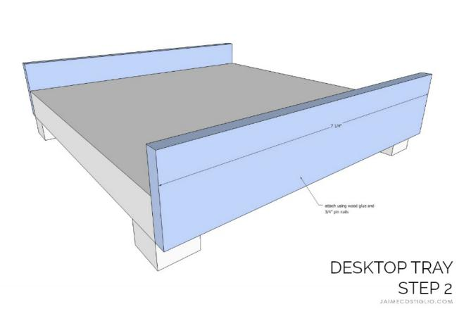
**Step 2:** Attach the short sides to the base using wood glue and 3/4" pin nails.
